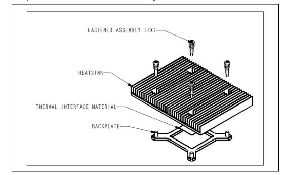
Figure 10. CompactPCI Reference Heatsink Assembly
